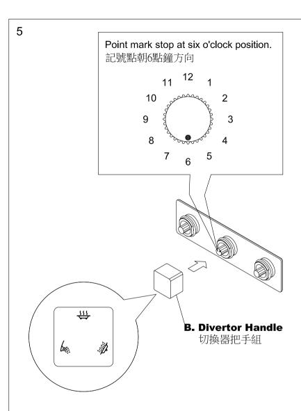
\* Keep the Mixer Valve straight ahead of you, then turning the **Divertor Spindle** until the Point mark stop at six o'clock position. Press **Divertor Handle** onto valve spindle until heard a click sound. 面對切換器中心栓,轉動中心栓,使記號點朝向6點鐘方向。將切換器把手依圖示方向組入中心栓,壓到底之後會有喀噠聲,表示安裝完成。
