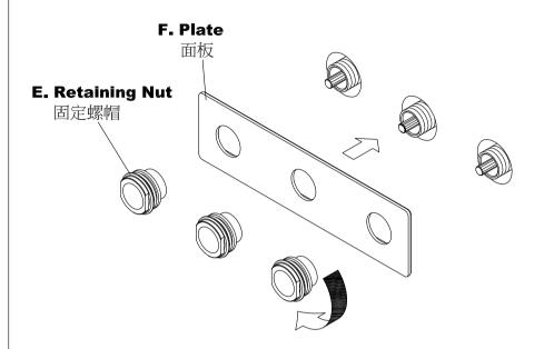
\* Fix the **Plate** against wall with **Retaining Nut**.
