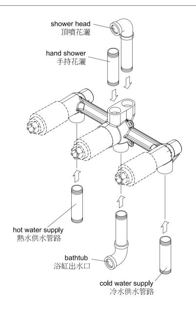
\* Install hot and cold water supply pipes and outlet.
