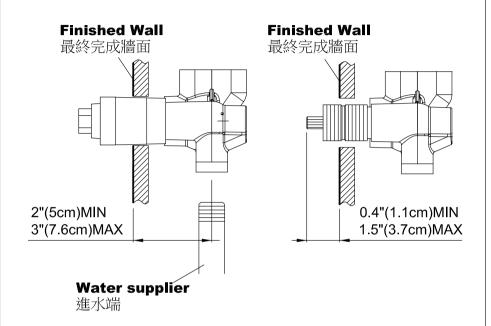
\* Connect hot and cold supplies pipes to the valve body, so they are between 2"(5cm) minmum and 3"(7.6cm) maximum from the finished wall; or keep the distance be 0.4" (1.1cm) to 1.5" (3.7cm) between top of cartridge and **Finished Wall** for necessary conditions.
