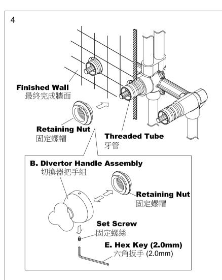
\* Disassemble the **Retaining Nut** from **Divertor Handle Assembly** with **Hex Key (2.0mm)**, then thread the **Retaining Nut** onto central **Threaded Tube** until it tighten against finished wall.
