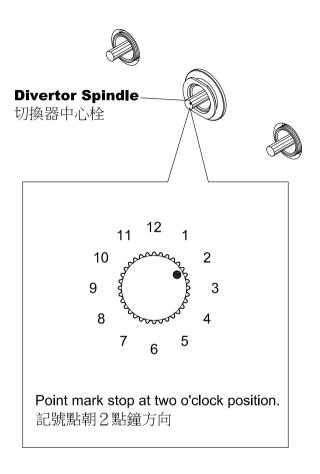
\* Keep the Mixer Valve straight ahead of you, then turning the **Divertor Spindle** until the Point mark stop at two o'clock position.
