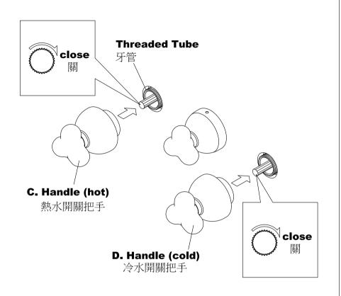
\* Turn **Hot Valve** and **Cold Valve** clockwise to closed position before install the **Handle Assembly**. Press both hot and cold **Handle Assembly** onto valve spindle and securely hand tighten the **Handle Assembly** against finished wall.
