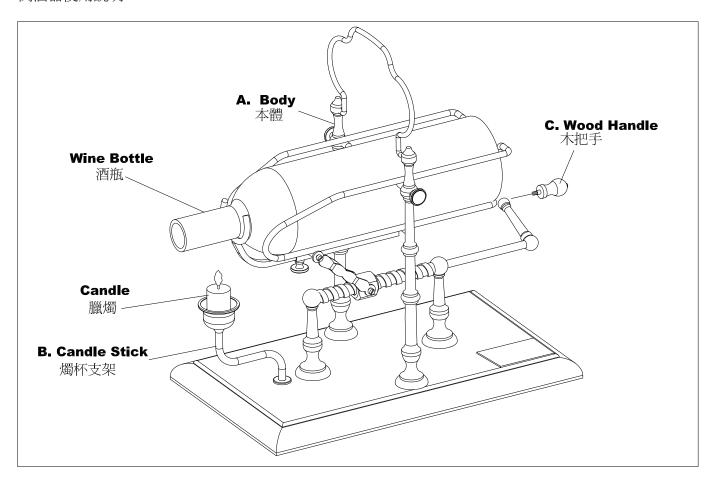
1. Hand-tighten Wood Handle into **Body**.
