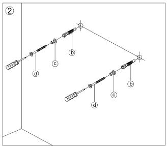
Using a 6mm drill-bit, drill the holes at marked positions to depth of 4cm. Insert the **Plastic Anchors** to the holes on the wall, put the **Screws** through the **Brackets**, then screw into the **Plastic Anchors**.
