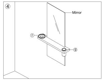
Put the **Soap Dish** and **Tumbler** on the **Woodle Shelf** as shown in figure #4. 樂門皇報和滅口杯放置平台上,完成安裝程序.
