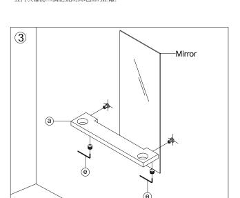
Use the **Hex Key** to lossen the **Set Screws** from the bottom of **Wooden Shelf**, slide the **Wooden Shelf** over the **Bracket** and tighten **Set Screws** as shown in figure #3. 用随附六角板手先鬆開平台下方的埋頭螺絲,使平台能順利套進固定基座後,再鎖緊下方的埋頭螺絲,
