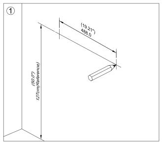
Mark 2 drill hole locations with a pencil on fixed dimension height position as shown in figure #1.
