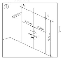
Mark two vertical lines A & B both sides 12.5cm from the center of drain outlet.
